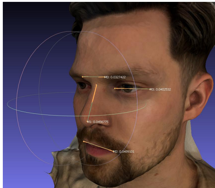
Inspection measurements of 3D scan done by COMPOACC
